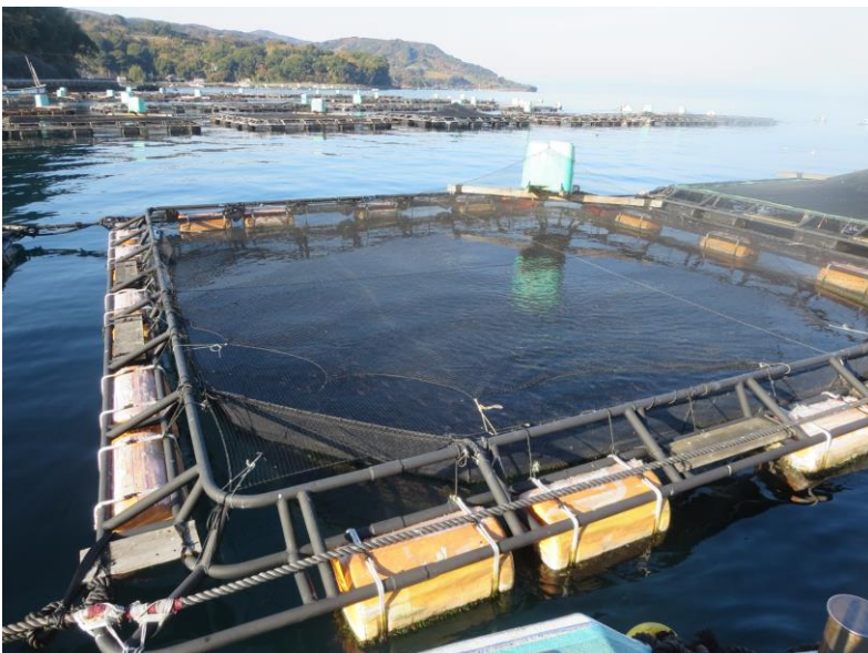
Foaming (polylactic acid) float under verification test in aquaculture cage
